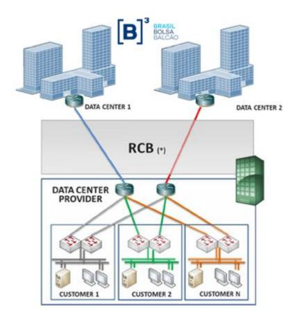
\* Links can be installed in one or more data centers on the data center provider's side, varying according to its structure.
