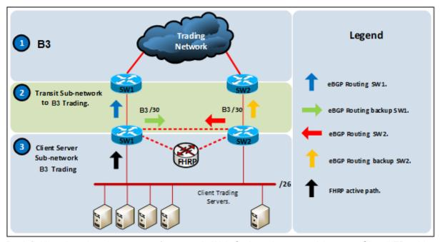
By definition, there is only one way of access via Web Co-Location, comprising two 1Gbps UTP cables. Each cable is connected to a different device at B3's data center to assure high availability of physical resources and network equipment.
