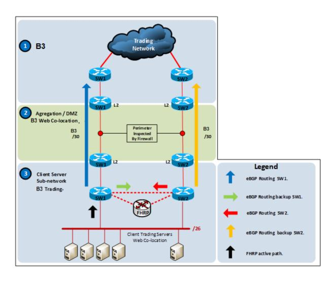
From the logical standpoint, the two connections to the trading bridge networks are point-to-point with IP addressing parameters supplied by B3 and /30 netmasks. The BGP protocol configuration is enabled on the bridging perimeter for connecting the institution's environment to B3B3's trading network.
