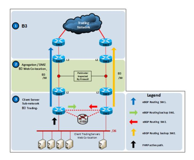
From the logical standpoint, the two connections to the trading bridge networks are point-to-point with IP addressing parameters supplied by B3 and /30 netmasks. The BGP protocol configuration is enabled on the bridging perimeter for connecting the institution's environment to B3B3's trading network.
