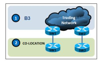
By definition, there is only one way of access via LAN Co-Location, comprising two pairs of 10Gbps multimode optical fiber cables. Each pair of optical fiber cable is connected to a different device in B3's data center to assure high availability of physical resources and network equipment.
