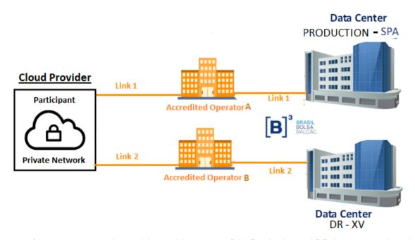
This way of access connects the participant with access to B3's Production and DR data centers through two different operators. It is also recommended that the links be connected to different POPs from the cloud provider.
