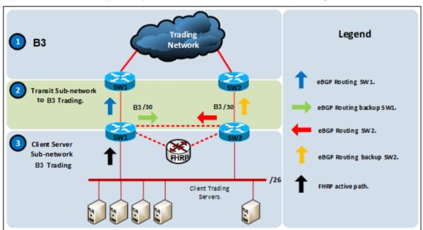
Each cable is connected to a different device at B3's data center to assure high availability of physical resources and network equipment.
