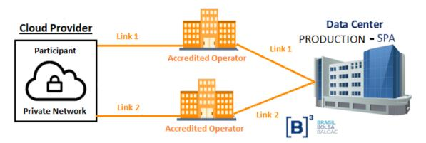
This way of access connects the participant's private network with high availability through two links to B3's production data center, each link being received on one of the two RCB edge routers
