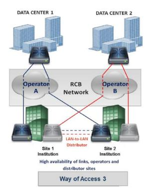
In this configuration, each of the institution's sites has two links, one to Data Center 1 and another to Data Center 2. Links for the same sites must be provided by different operators. This is the most complete configuration: in addition to redundant access to B3's technology infrastructure and to the operator's backbone, it allows institutions to operate via an adjacent active site if one of their sites is totally unavailable.
