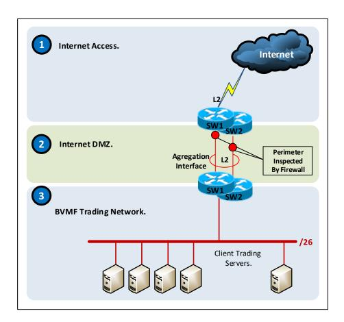
From a logical standpoint, the participant's internet connection link switch will run a layer 2 configuration, which will pass through a firewall and take this access to the participant's trading rack. In this perimeter, the internet inbound and outbound communication ports will be restricted.
