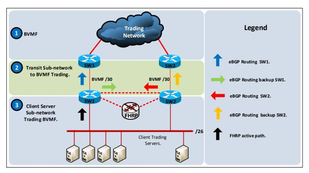
From a logical standpoint, the two connections to the trading bridge networks are point-to-point with IP addressing parameters supplied by BM&FBOVESPA and /30 netmasks. The BGP protocol configuration is enabled on the bridging perimeter for connecting the institution's environment to BM&FBOVESPA's trading network.
