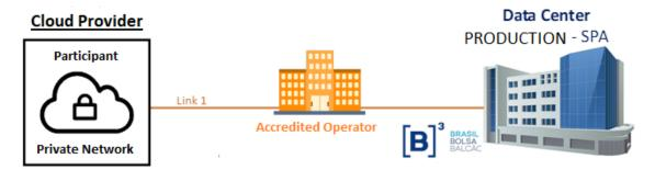
This way of access connects the participant's private cloud network via a single link to B3's production data center, on one of RCB's edge routers.
