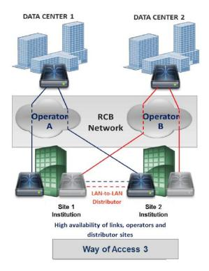
In this configuration, each of the institution's sites has two links, one to Data Center 1 and another to Data Center 2. Links for the same sites must be provided by different operators. This is the most complete configuration: in addition to redundant access to BM&FBOVESPA's technology infrastructure and to the operator's backbone, it allows institutions to operate via an adjacent active site if one of their sites is totally unavailable.
