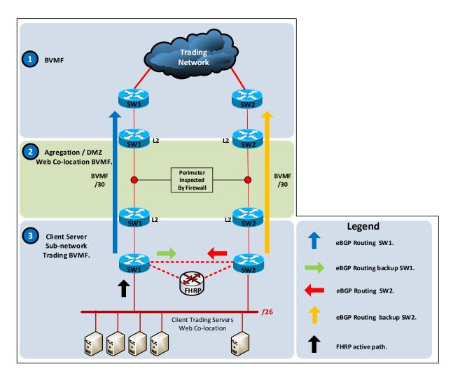
From the logical standpoint, the two connections to the trading bridge networks are point-to-point with IP addressing parameters supplied by BM&FBOVESPA and /30 netmasks. The BGP protocol configuration is enabled on the bridging perimeter for connecting the institution's environment to BM&FBOVESPA's trading network.
