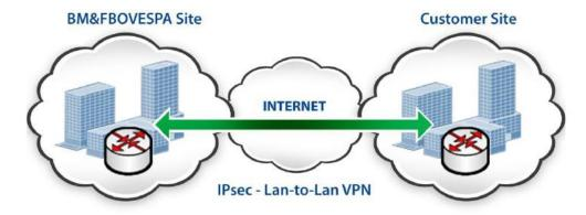
LAN-to-LAN VPN access is available for all the systems and environments listed in Annex 1, guaranteeing greater scalability for institutions. Access is authorized only using the address block supplied by BM&FBOVESPA. Other network addresses may have to be translated to the address supplied using NAT. In this way of access, customers are responsible for equipment configuration, management, internet access and security.
