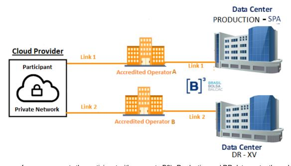
This way of access connects the participant with access to B3's Production and DR data center through two different operators. It is also recommended that the links be connected to different POPs from the cloud provider.
